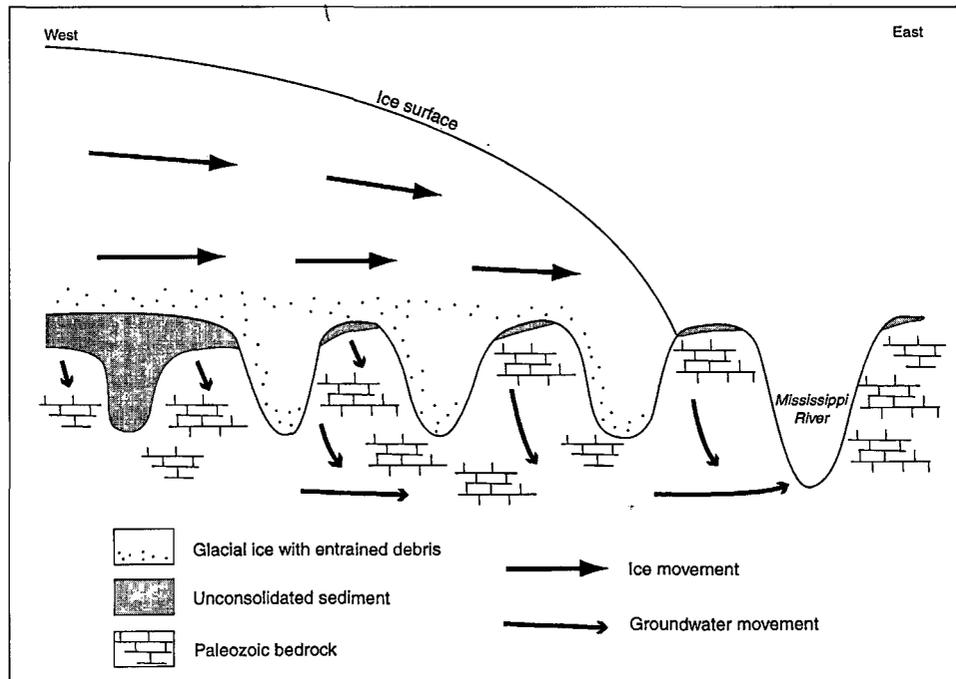
Figure 2. Schematic diagram showing proposed drainage of subglacial meltwater where ice sheet encroaches on the Paleozoic Plateau. Length of arrow on ground-water flowpaths indicates relative amount of subglacial meltwater draining into the bedrock.
