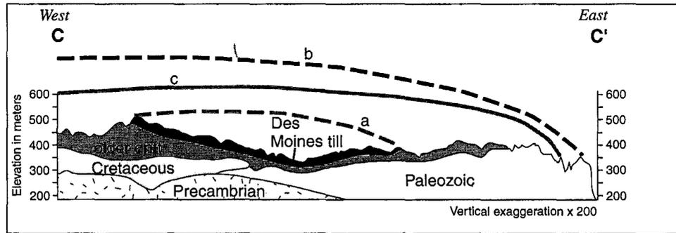
Figure 4. Topographic and generalized stratigraphic profile along the Iowa-Minnesota border (C-C' on Fig. 1) at latitude 43°30'N, and hypothetical ice profiles. Vertical exaggeration  $\times 200$ . a, Upper surface of Des Moines lobe ice from Clark (1992); b, Maximum elevation of upper surface of ice during pre-Illinoian glacial maximum; c, "Intermediate" elevation of the upper surface of the ice during pre-Illinoian glacial maximum. See text for discussion of curves b and c.
